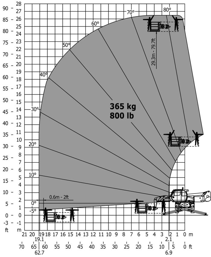
Rotation on lowered stabilisers with 365/1000 kg platform
