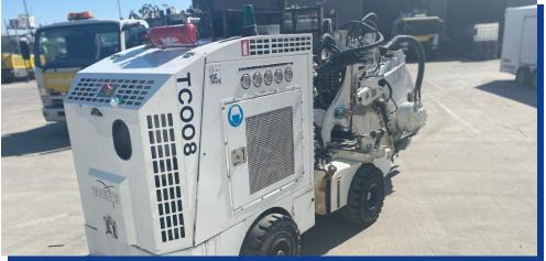
Thanks to its compact size the Marais SC2P wheeled sidecut allows cutting on sidewalks and can operate in narrow spaces, with limited disturbance to pedestrian and traffic during the works. It's a machine that assures less personnel needed on site, increases the safety and reduces the environmental impact.
